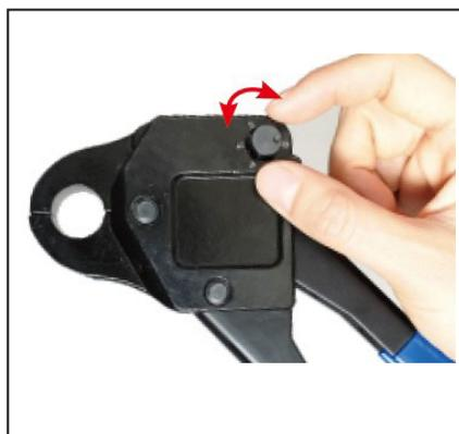
2. Push & rotate pin increase by single increment only.
